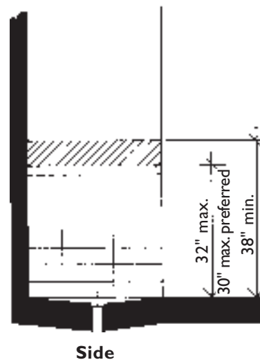
Minimum Reinforcing for Grab Bars in Showers
