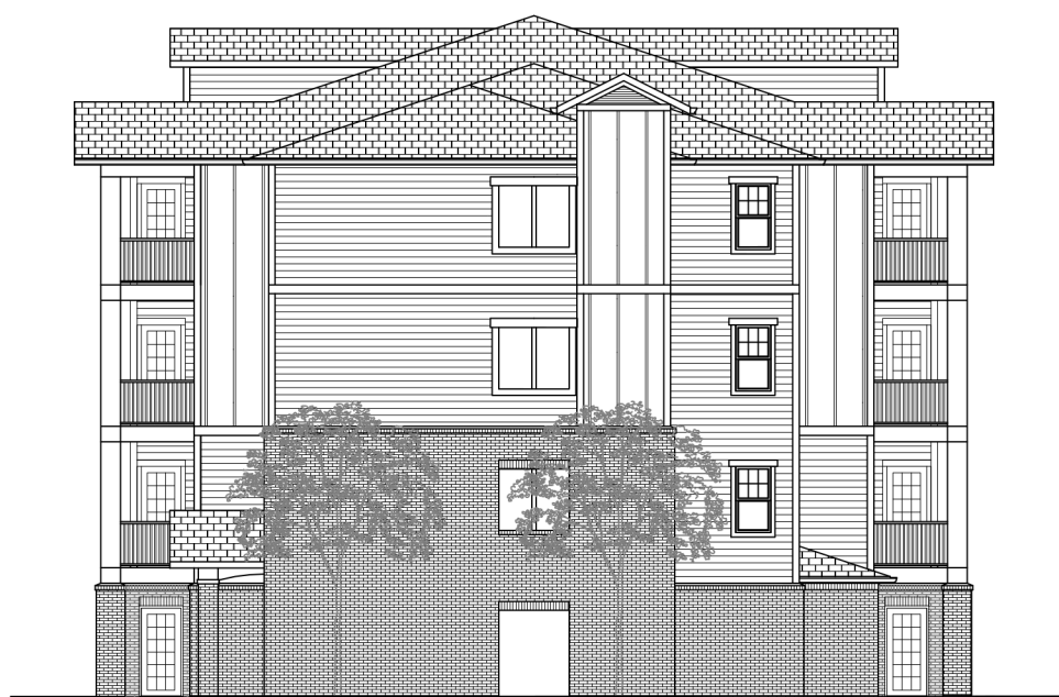
4 BUILDING #100 RIGHT ELEVATION 1/16" = 1'-0"
