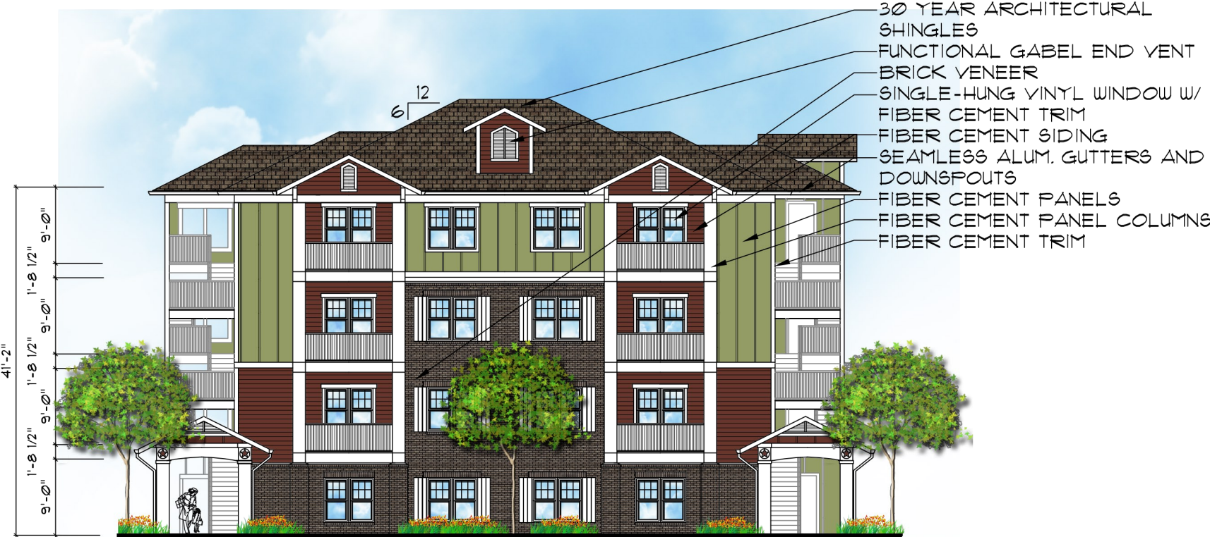
1 BUILDING #100 FRONT ELEVATION 1/16" = 1'-0"
